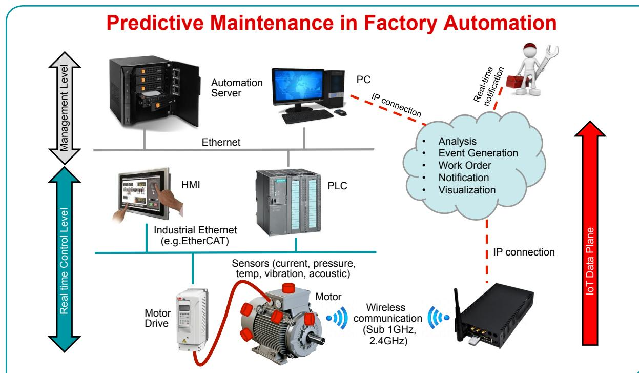
**Figure 1.** Predictive maintenance in factory automation.
