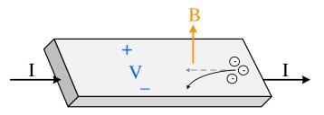
Figure 2. The Hall effect produces a measurable voltage proportional to the interacting electric current and magnetic field.
