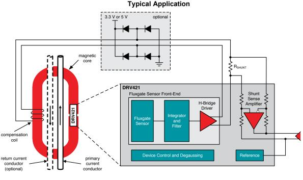
*Figure 4.* High-resolution DRV421 and DRV425 integrated fluxgate magnetic sensors simplify closed- and open-loop current-sensing designs.
