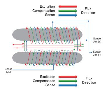
Figure 3. The Förster-type fluxgate includes two parallel magnetic cores and three sets of interwound solenoid coils.
