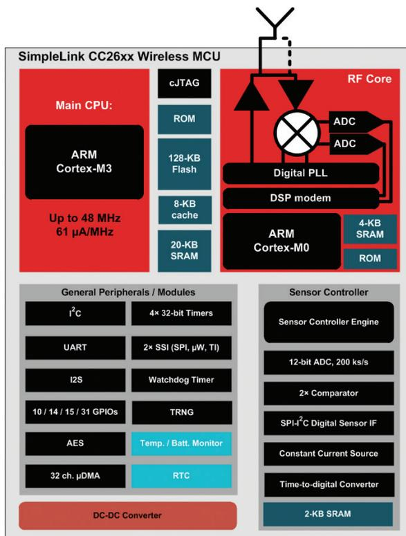
Figure 6. SimpleLink CC26xx wireless MCU functional diagram.
