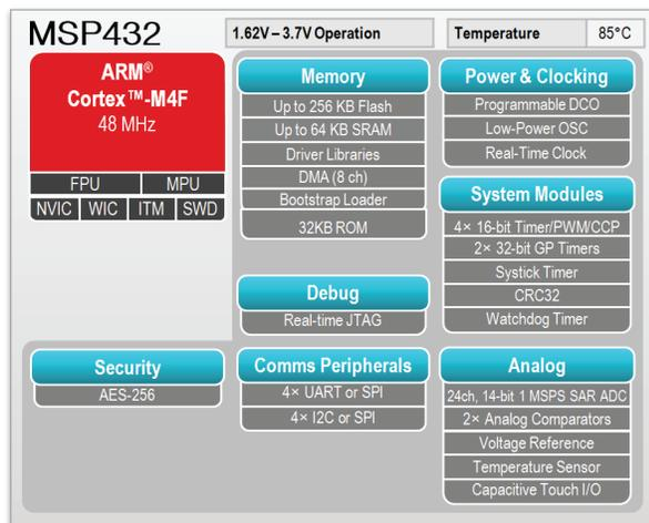
**Figure 3.** SimpleLink MSP432 MCU with 14-bit ADC.
