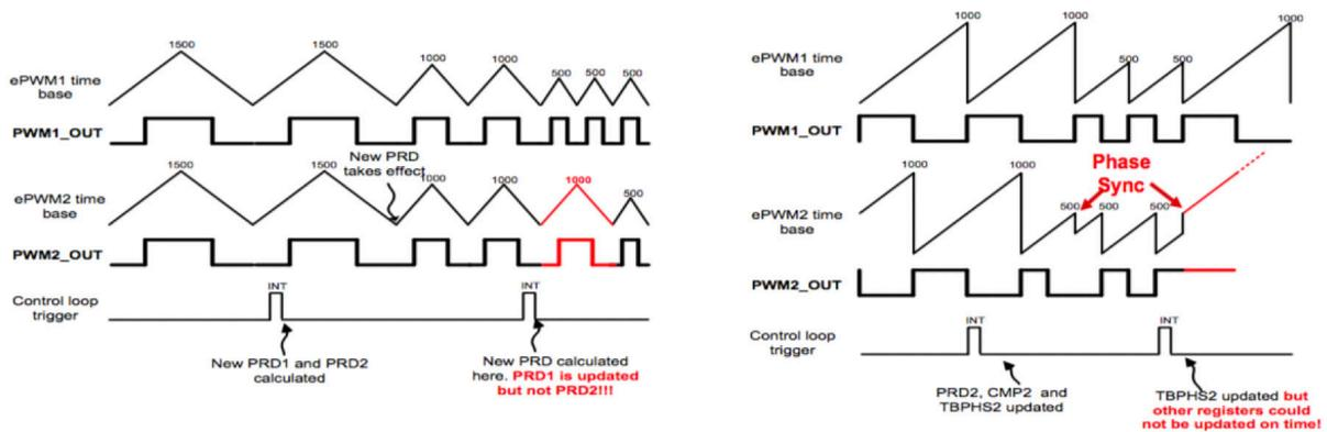
Figure 3. Challenges for variable-frequency PWM waveform generation.
