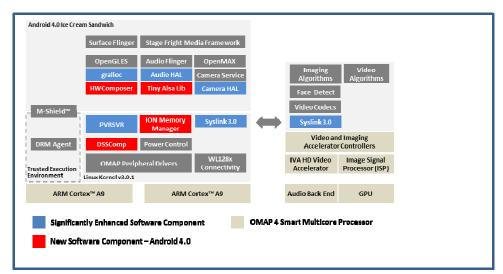
**Figure 1** - Android 4.0 OMAP 4 Board Support Package (A4O4 BSP) Architecture Overview (Selected Components)
