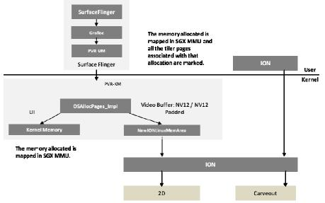
Figure 5 - Overview of Buffer Management Components in A4O4 BSP.
