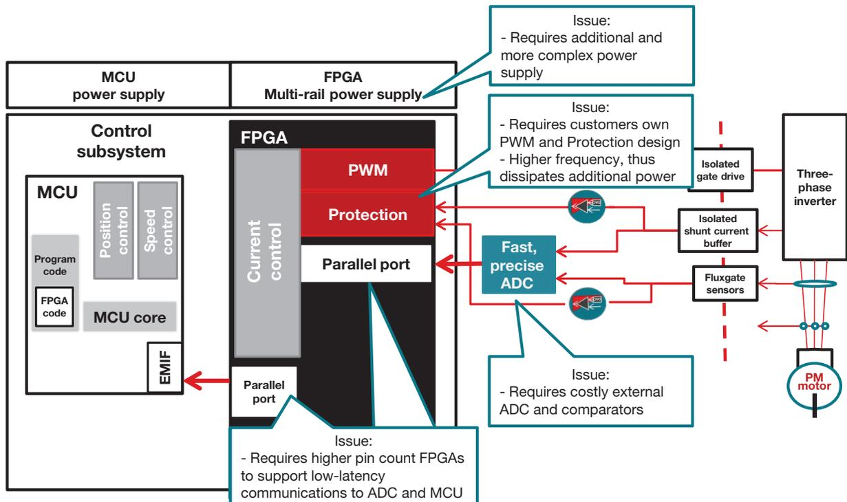
Figure 1. System challenges associated with FPGA-based current-loop control.
