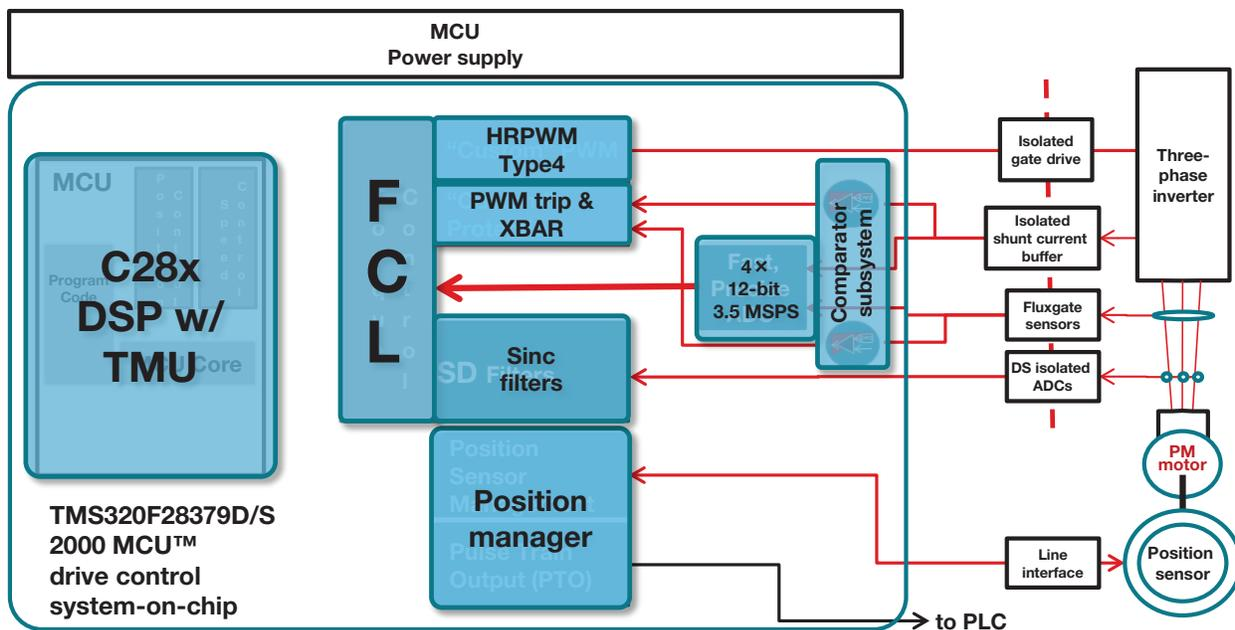
Figure 2. C2000 system integration for industrial drives.
