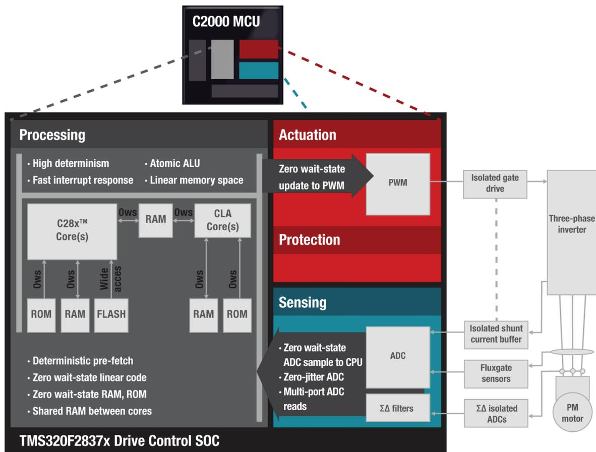
Figure 3. C2000 MCUs architecture for real time control.
