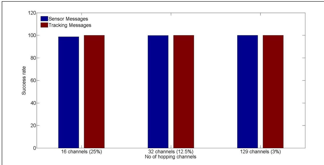
**Figure 6:** Robustness achieved using application level retransmissions
