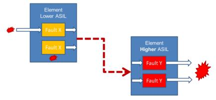
Figure 2. Example of Cascading Failure Causing Interference in Higher ASIL Safety Function
