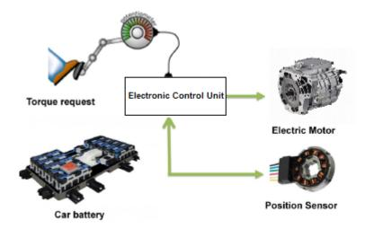
Figure 1. Electric Vehicle Traction Control System
