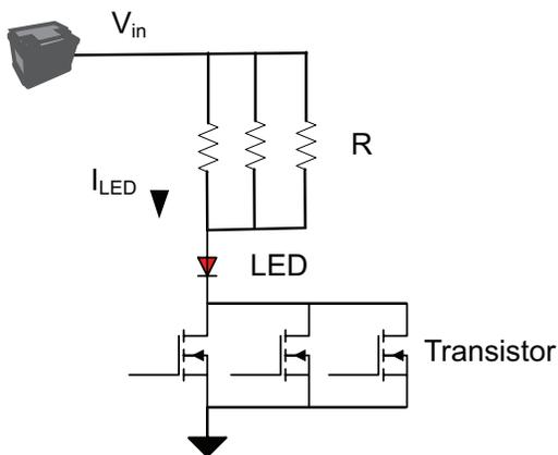
**Figure 9.** Discrete LED driver.
