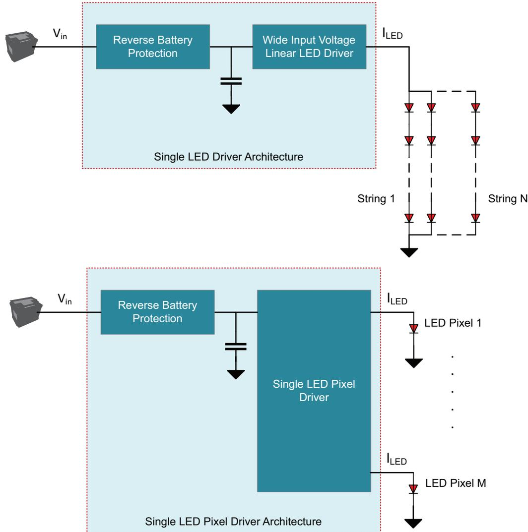
**Figure 5.** Controlling strings of LEDs with one LED driver vs. controlling each LED independently.
