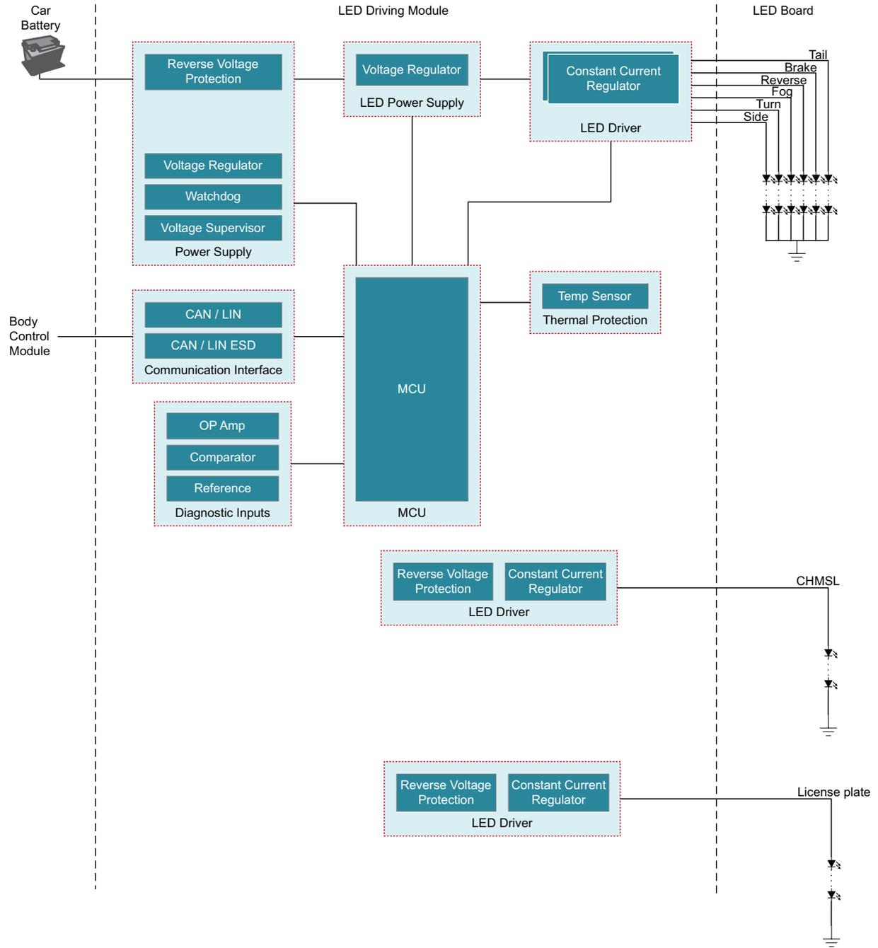
Figure 2. Block diagram of a rear light control module.
