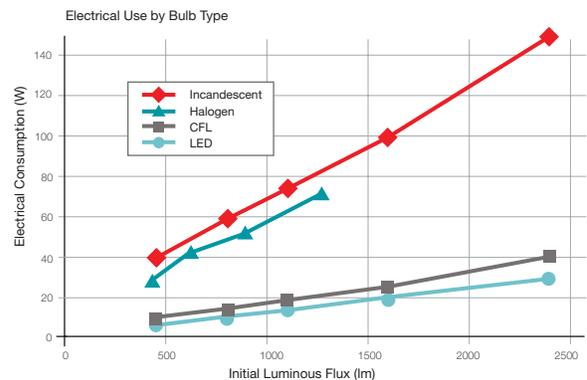
**Figure 4.** Efficiency of an LED light source vs. an incandescent bulb. (Source: [https://commons.wikimedia.org/wiki/File:Electricity\\_use\\_by\\_lightbulb\\_type.svg](https://commons.wikimedia.org/wiki/File:Electricity_use_by_lightbulb_type.svg))
