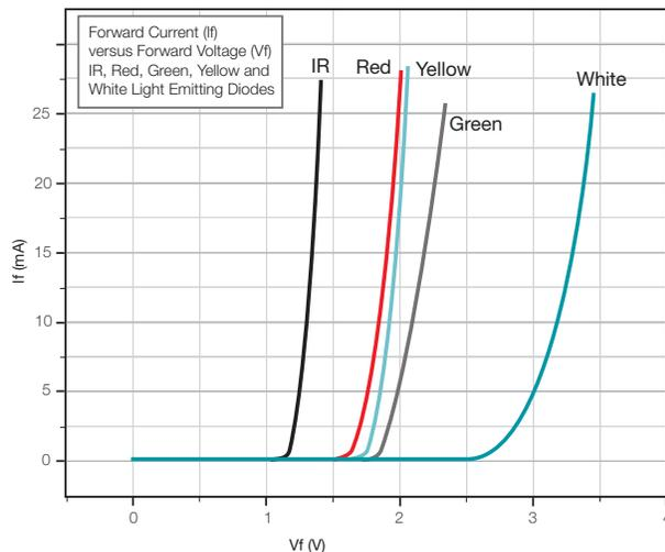
**Figure 3.** An LED's I-V curve. (Source: <http://lednique.com/current-voltage-relationships/iv-curves/>)
