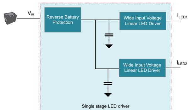
Figure 7. Single-stage LED driver.
