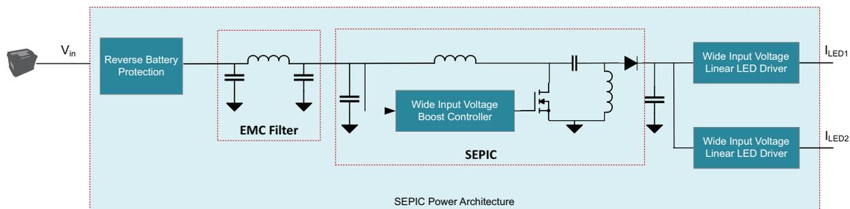
Figure 8. Dual-stage LED driver.
