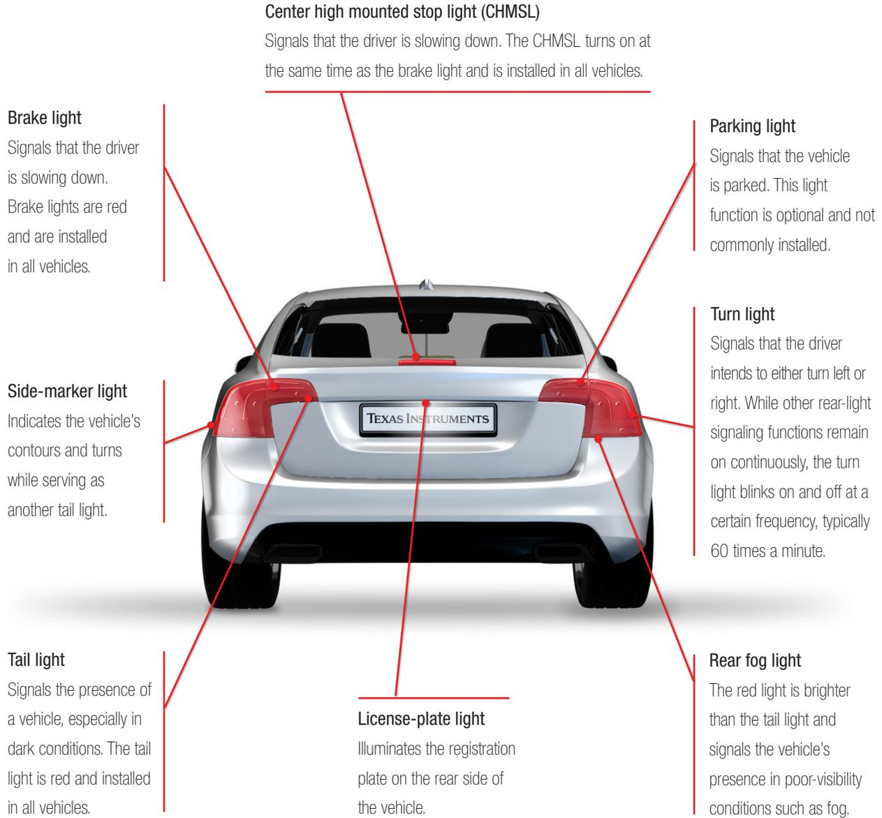
**Figure 1.** Components of a rear-lighting system.
