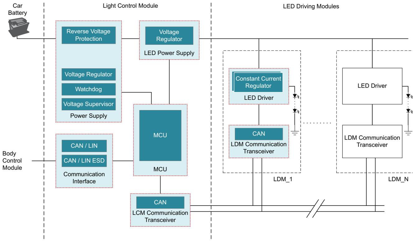
**Figure 6.** A digital interface LED driving module architecture for pixelated rear lights.
