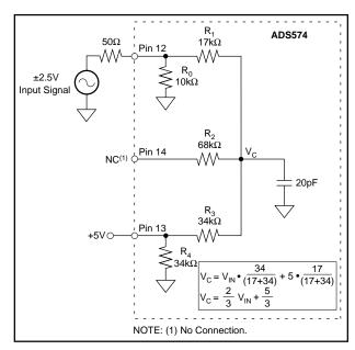
FIGURE 6. Connections for ±2.5V Input Range.
