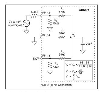
FIGURE 4. Connections for 0V to +5V Input Range.
