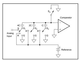
FIGURE 2. Simplified 3-bit Switched Capacitor Array A/D.
