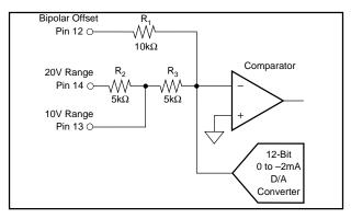
FIGURE 1. Traditional ADC574 Input Structure.
