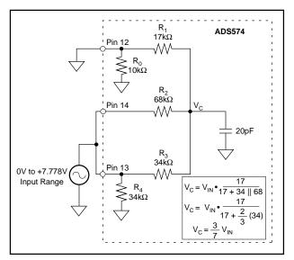
FIGURE 7. Connections for 0V to +7.778V Input Range.
