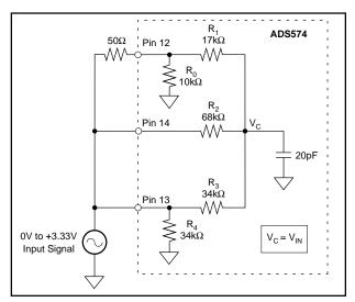
FIGURE 5. Connections for 0V to +3.33V Input Range.
