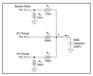
FIGURE 3. ADS574 Input Structure.
