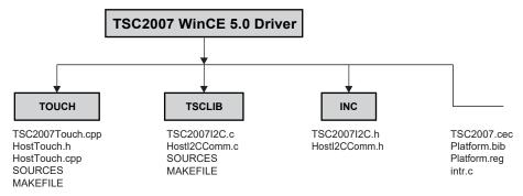
Figure 2. TSC2007 WinCE 5.0 Driver Files with I<sup>2</sup>C Control Interface
