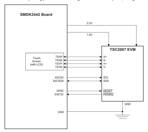
Figure 1. TSC2007 Connection to SC32442 Application Processor
