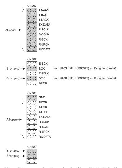
Figure 5-2. Jumper Configuration for Slave Mode (Default)
