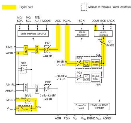
Figure A-4. Mono Microphone Input (AIN1L, +20 dB)
