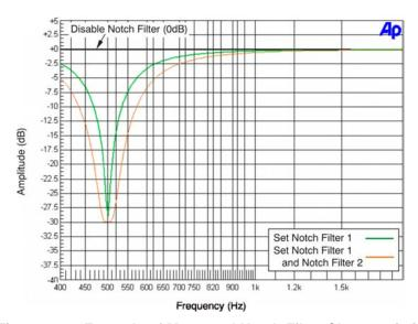
Figure 3-12. Example of Measured Notch Filter Characteristic
