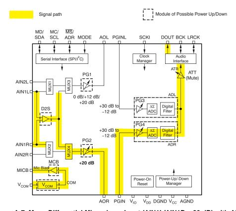
Figure A-7. Mono Differential Microphone Input (AIN1L/AIN1R, +20 dB) with ALC
