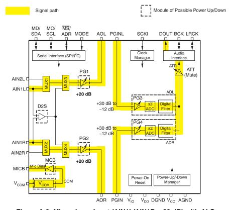
Figure A-3. Microphone Input (AIN1L/AIN1R, +20 dB) with ALC
