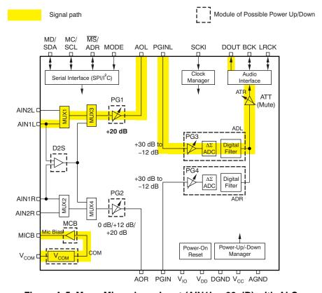
Figure A-5. Mono Microphone Input (AIN1L, +20 dB) with ALC
