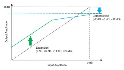
Figure 3-8. ALC Compression and Expansion Characteristics
