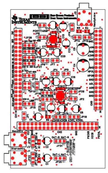
Figure 6-3. DEM-PCM1870RHF/1774RGP-A Board Layout—Silkscreen Side
