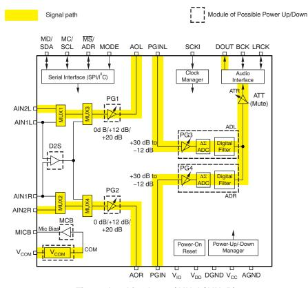
Figure A-1. Line Input (AIN2L/AIN2R)
