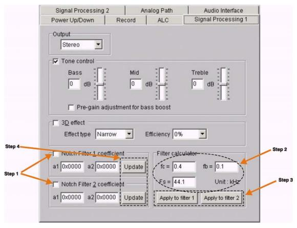
Figure 3-9. Signal Processing 1 Function Menu Tab
