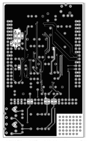
Figure 6-7. DEM-PCM1870RHF/1774RGP-A Board Layout—Solder Side
