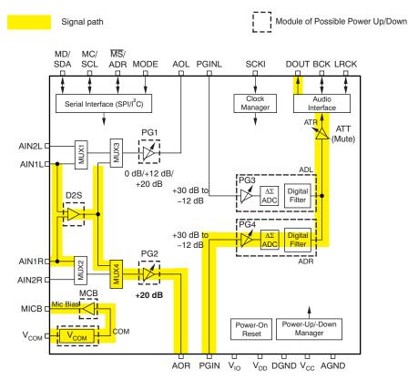
Figure A-6. Mono Differential Microphone Input (AIN1L/AIN1R, +20 dB)
