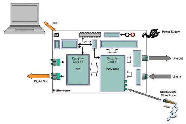
Figure 1-2. DEM-DAI1870 EVM System Diagram
