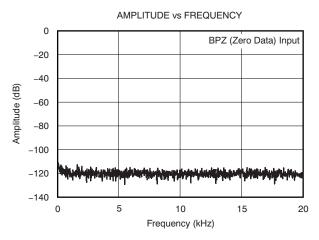
Figure 5-9. ADC Amplitude vs Frequency Result: BPZ (Zero Data) Input
