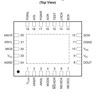
Figure 1-1. PCM1870 Pin Assignments
