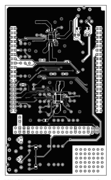
Figure 6-4. DEM-PCM1870RHF/1774RGP-A Board Layout—Component Side
