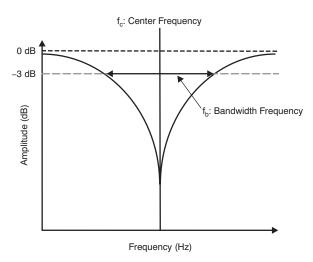
Figure 3-11. Notch Filter Characteristic Model
