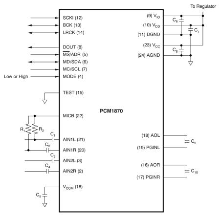
Figure 5-10. Basic Connection Diagram
