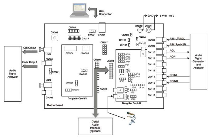
Figure 2-2. EVM and External Equipment Connections
