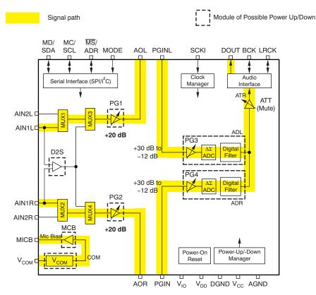
Figure A-2. Microphone Input (AIN1L/AIN1R, +20 dB)
