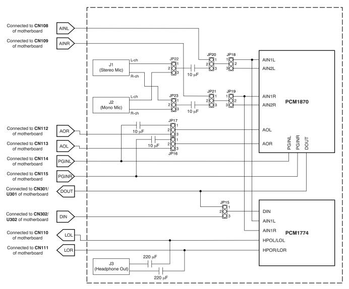
Figure 4-2. Analog Input/Output Configuration (Daughter Card #1)
