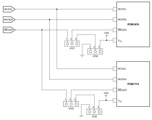
Figure 4-3. MS/ADR Control Configuration for I<sup>2</sup>C Communication (Daughter Card #1)
