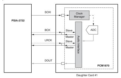
Figure 5-5. Combined Master and Slave Mode Configuration with SYS-2722
