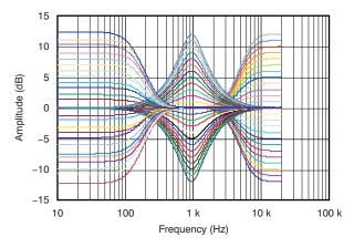
Figure 3-10. Three-Band Tone Control (Bass, Mid, Treble)
