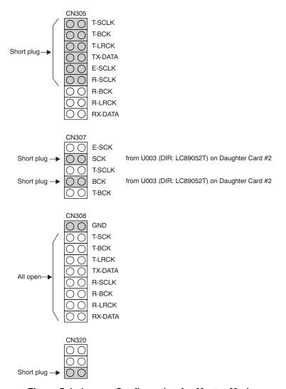
Figure 5-4. Jumper Configuration for Master Mode
