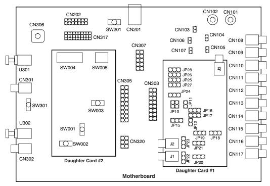
Note: Silkscreen symbol CN320 is not printed on the motherboard, but it is located in the position described.
