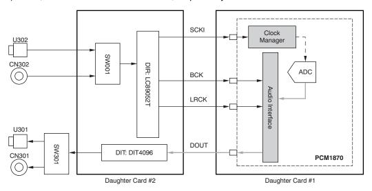
Figure 5-1. Slave Mode Configuration With SYS-2722
