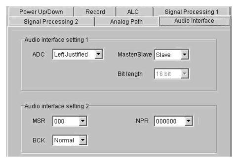
Figure 3-16. Audio Interface Function Menu Tab
