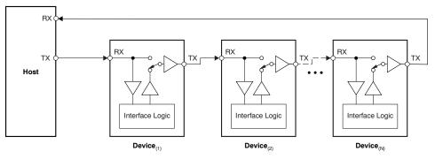
Figure 10. TMP104 Daisy-Chain: Bus Status at Start of Address Assignment
