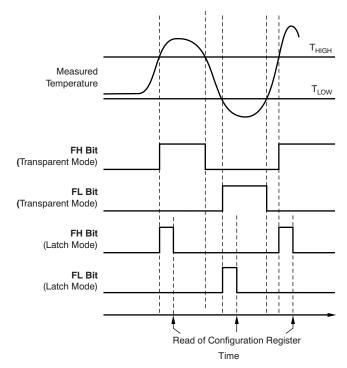
Figure 13. Temperature Flag Functional Diagram
