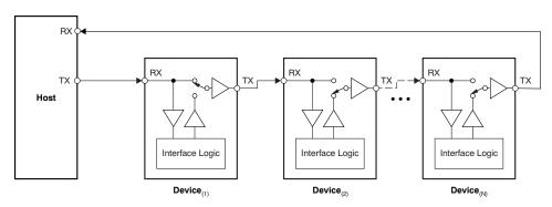
Figure 11. TMP104 Daisy-Chain: Bus Status After First Device Address Assignment
