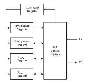
Figure 8. Internal Register Structure
