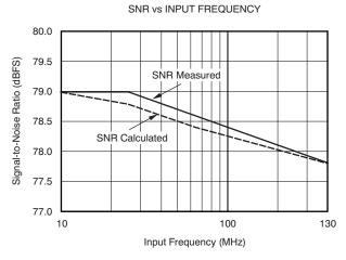
Figure 3. Measured vs. Predicted SNR Performance Over Input Frequency
