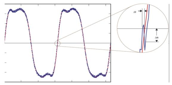
Figure 4. Sampling Error Caused by Thermal Noise Component
