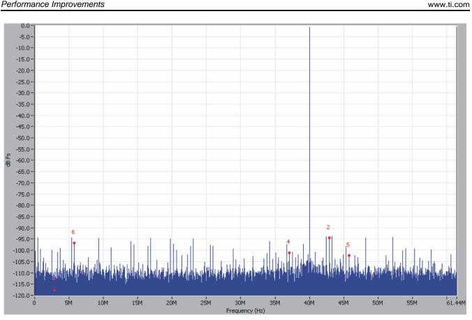
Figure 12. Spectral Performance with the CDCE72010 Clock Source at 30-MHz IF Input
