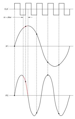
Figure 2. SNR Degradation as a Result of Jitter for Different IF Input Signals
