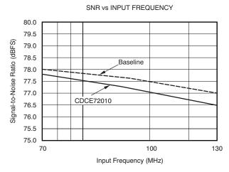
Figure 15. SNR Performance vs IF Input Frequency
