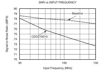
Figure 11. SNR Performance vs IF Input Frequency
