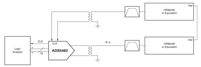
Figure 9. ADC Evaluation Test Setup (Baseline)
