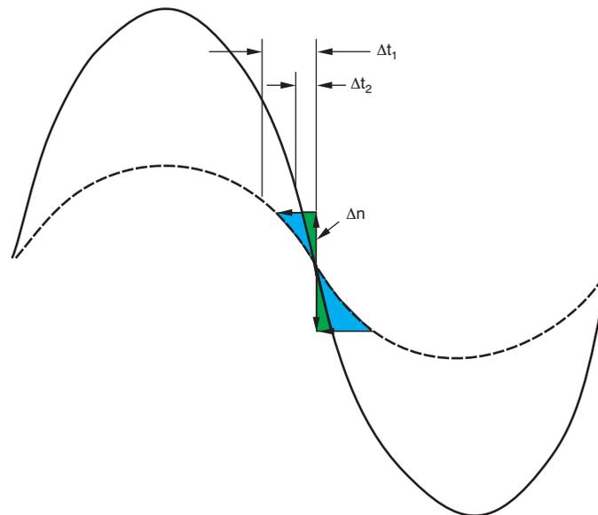
**Figure 7. Thermal Noise Effect for Different Amplitude Sinusoids**
