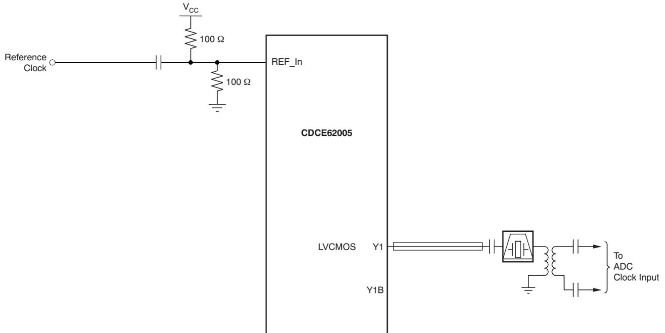
**Figure 9. CDCE62005 Interface to ADCs for High IF Input Frequencies**
