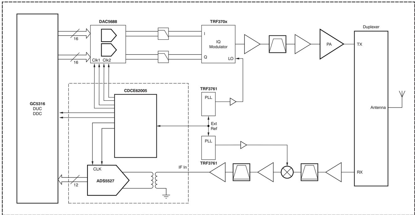
Figure 1. ADS5527 with CDCE62005 Clocking Solution within a Typical Base Station Application
