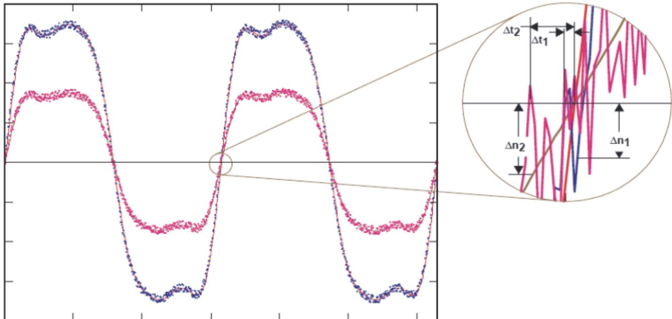
**Figure 6. Thermal Noise Effect for Different Slope Clock Signals**
