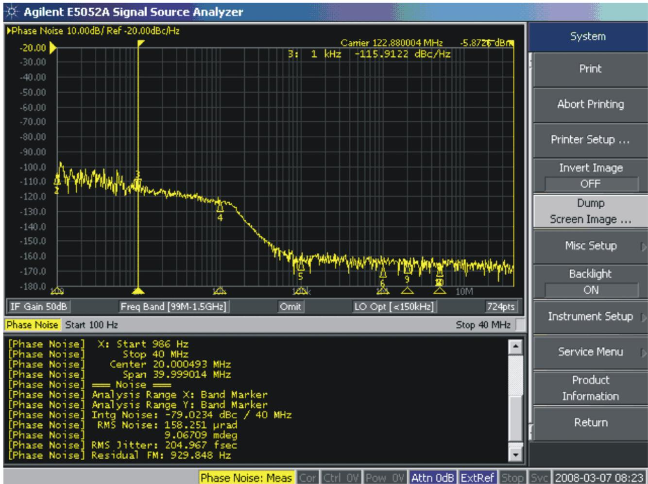
Figure 15. CDCE62005 122.88-MHz Filtered LVCMOS Output Phase Noise
