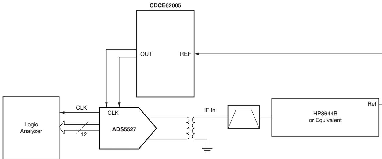
Figure 11. ADC Evaluation Test Setup with the CDCE62005 Clock Source
