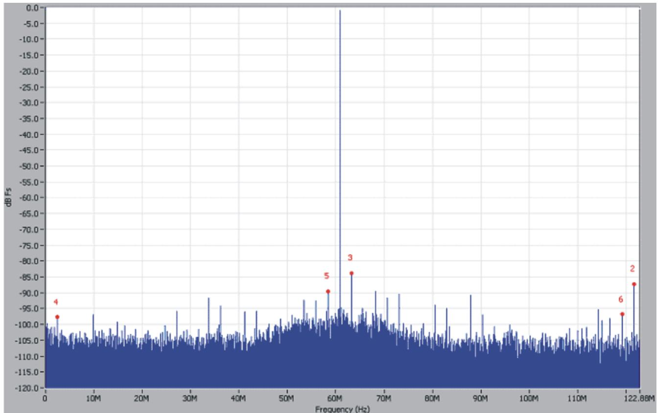
**Figure 13. Spectral Performance with the CDCE62005 Clock Source at 5-MHz IF Input**
