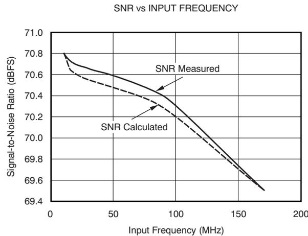
**Figure 4. Measured vs Predicted SNR Performance Over Input Frequency**
