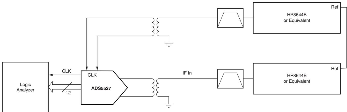
**Figure 10. ADC Evaluation Test Setup (Baseline)**
