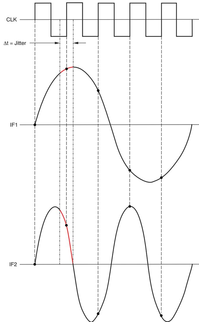
**Figure 3. SNR Degradation Caused by Jitter for Different IF Input Signals**
