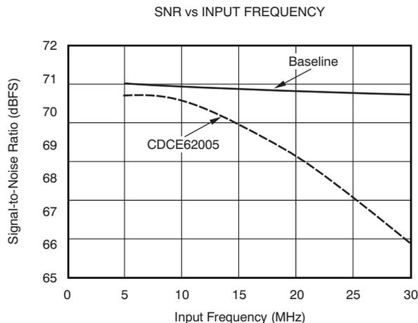
Figure 12. SNR Performance vs IF Input Frequency
