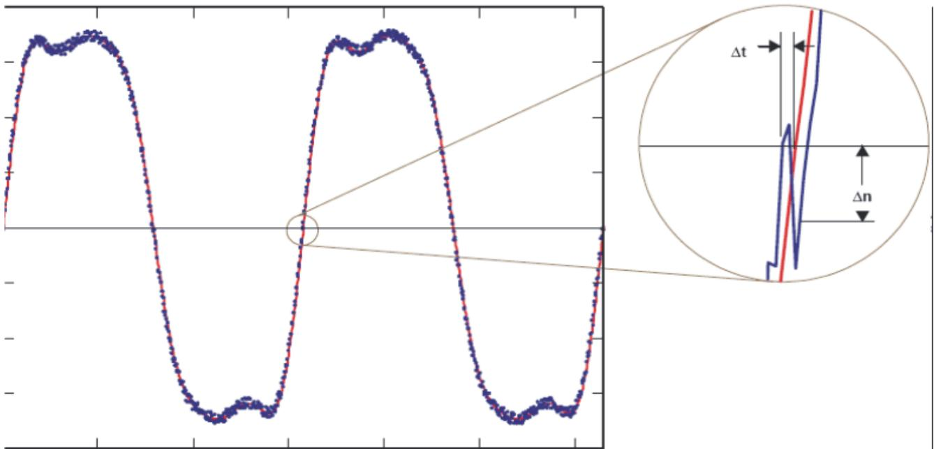
**Figure 5. Sampling Error Caused by Thermal Noise Component**
