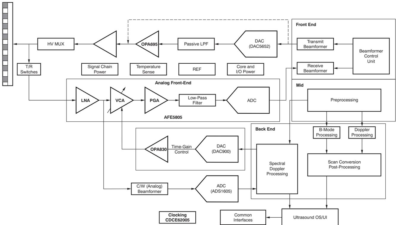
Figure 2. AFE5805 with CDCE62005 Clocking Solution within a Typical Medical Ultrasound Application
