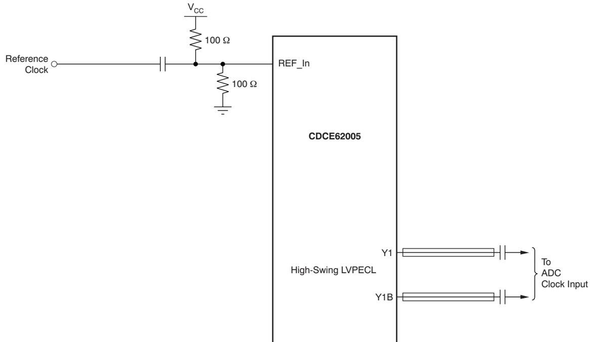
Figure 8. CDCE62005 Interface to ADCs for Low IF Input Frequencies
