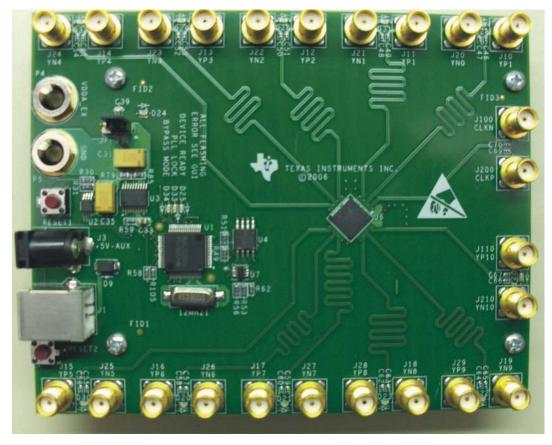
Figure 1. CDCL6010 Evaluation Board
