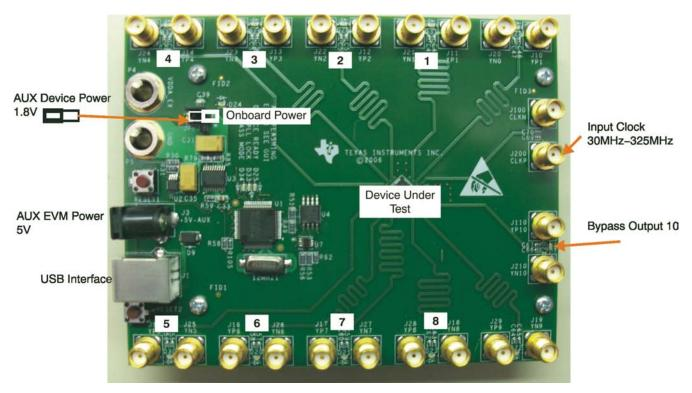
Figure 2. CDCL6010EVM Controls and Connectors
