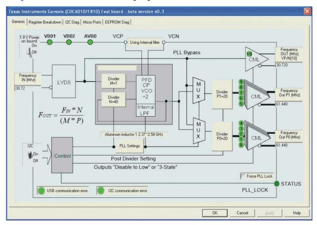
Figure 7. TI Genesis Software GUI
