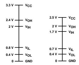
Figure 1. 3.3-V and 2.5-V V<sub>CC</sub> Thresholds
