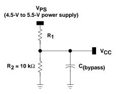
Note:  $C_{(bypass)} = 0.1 \text{ to } 0.01 \,\mu\text{F}$
