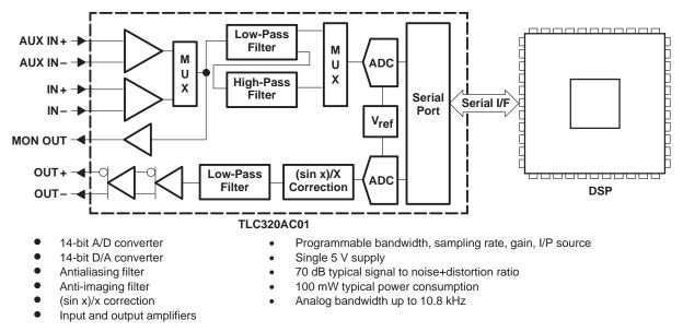
Figure 1. TLC320AC01 Analog Interface for DSP
