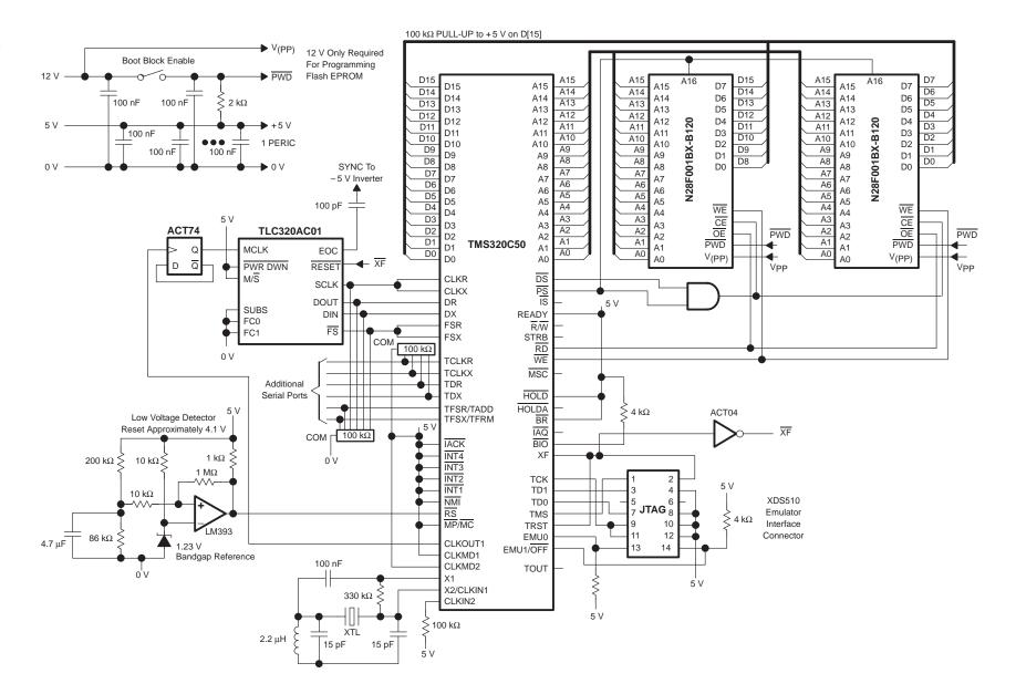
Figure 9. TLC320AC01 to TMS320C50 Hardware Schematic
