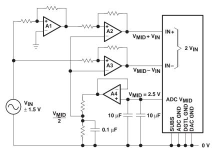
Figure 4. 0-V Referenced Input Circuit
