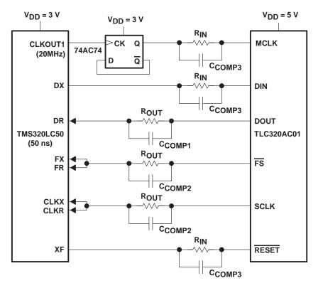
Figure 10. Interfacing to 3-V DSP
