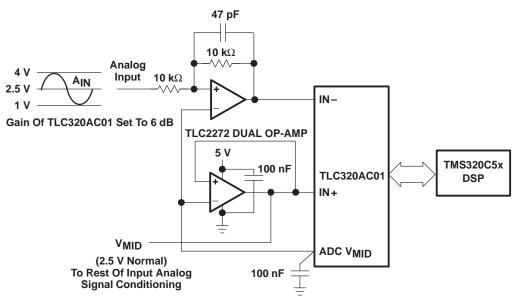
Figure 3. V<sub>MID</sub> Referenced Input Circuit
