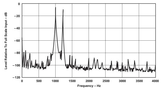
Figure 2. ADC Noise and Distortion Measurement
