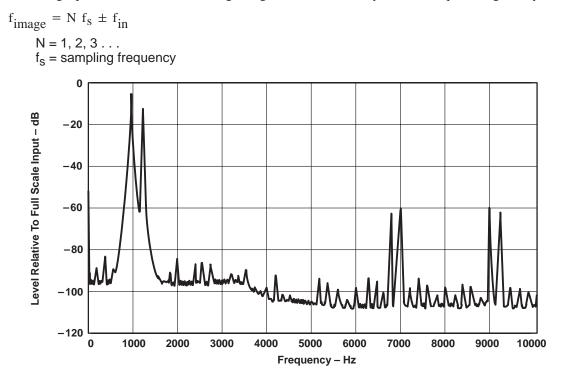
Figure 6. DAC Noise and Distortion Measurements
