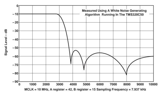
Figure 12. DAC Channel Frequency Response
