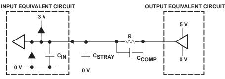
Figure 11. Interfacing to 3-V DSP – Component Values
