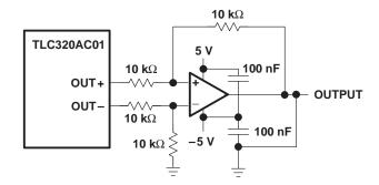
Figure 7. Differential to Single Ended Output Circuit
