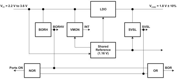
NOTE: BORHV is active-high polarity (1 = V<sub>CC</sub> domain is in reset). SVSL is active-high polarity (1 = V<sub>CORE</sub> domain is in reset).
