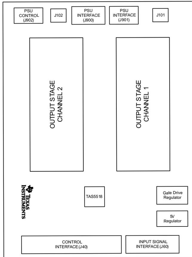
**Figure 2. Physical Structure for the TAS5518-5261K2EVM (Approximate Layout)**
