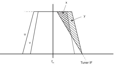
Figure 5. UV Frequency Spectrum (u Bandwidth Greater Than v)
