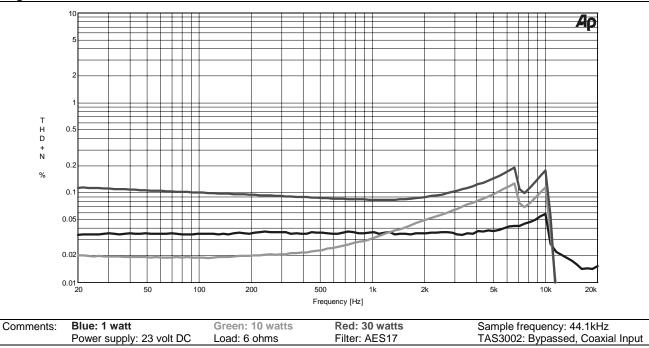
Note: THD+N at high frequencies depends on the output-filter coil material.
