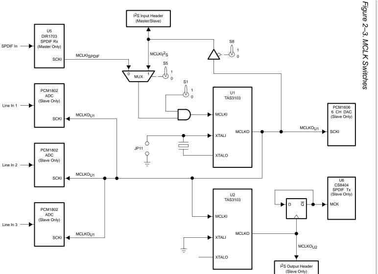
If TAS3103–U1 is the source of MCLK and this clock is being supplied to the I<sup>2</sup>S input port, S8 must be set to L. The architecture of the TAS3103 allows it to be the source of MCLK and yet be slaved to external SCLK and LRCLK clocks. This means that TAS3103–U1 can supply MCLK to an external device connected to the I<sup>2</sup>S input port and operate as a slave using SCLK and LRCLK.
