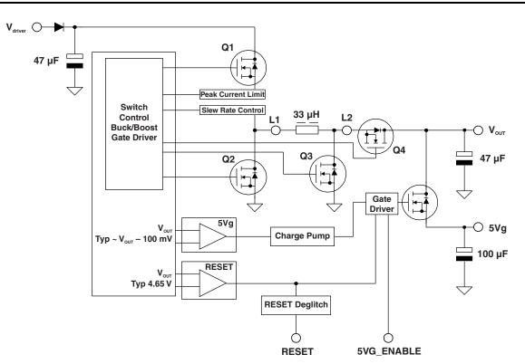
Figure 8. Primary and Secondary Output Voltage Terminals
