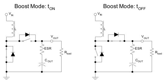
Figure 5. Equivalent Schematics - Boost Mode
