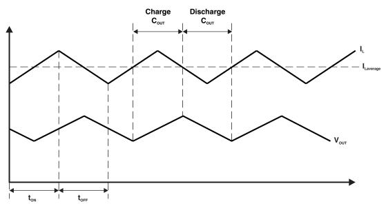
Figure 4. Ideal Buck Converter, Continuous Conduction,  $I_L$  and  $V_{OUT}$  vs Time
