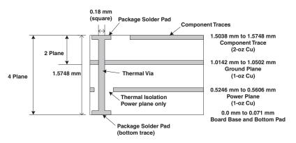
Figure 11. Thermal Vias With Multilayer Board (Side View)
