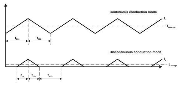
Figure 2. Continuous and Discontinuous Conduction Modes
