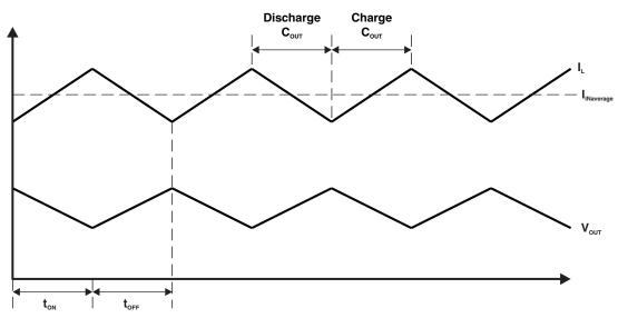
Figure 6. Ideal Boost Converter, Continuous Conduction,  $I_{\text{L}}$  and  $V_{\text{out}}$  vs Time
