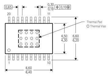
Figure 10. PWP Package With Thermal Pad
