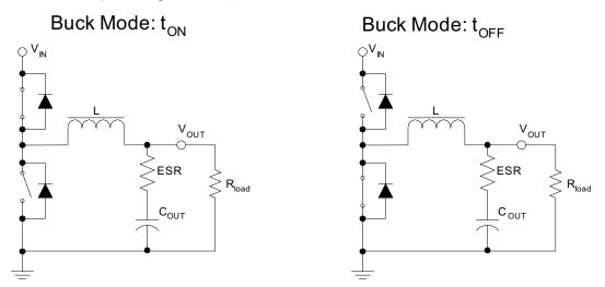
Figure 3. Equivalent Schematics – Buck Mode
