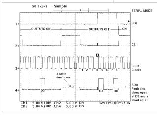
Figure 5. Open/Short-Fault Conditions Note that FLT0 occurs in the second byte of data.
