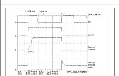
Figure 4a. Power During On Time
