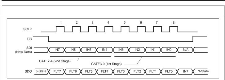
Figure 10. 8-Bit Serial Word Operation
