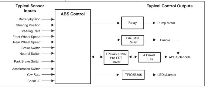
Figure 1. ABS Control Block Diagram
