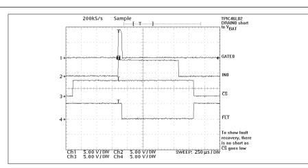
Figure 7. Fault Clears
