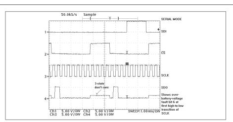
Figure 9. Under-Battery Fault Condition
