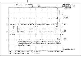
Figure 6. Fault is Captured
