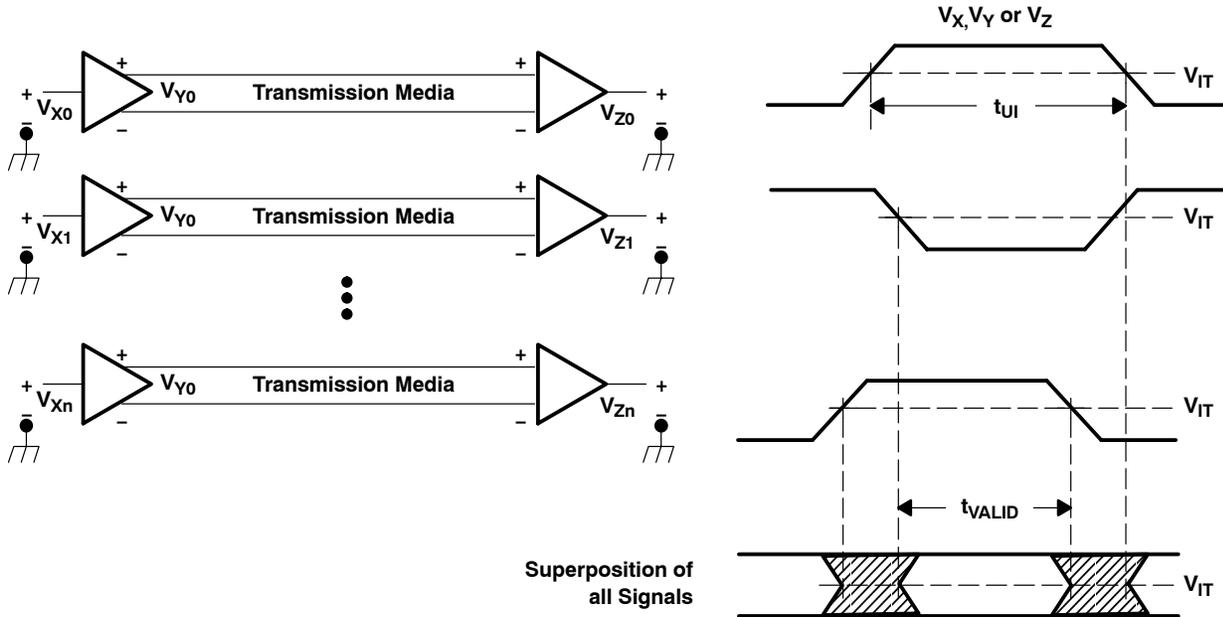
**Figure 2. Parallel Operation of Data Interchange Circuits**
