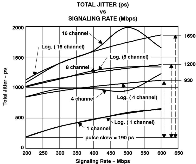
Figure 5. Jitter vs Signaling Rate and Number of Channels
