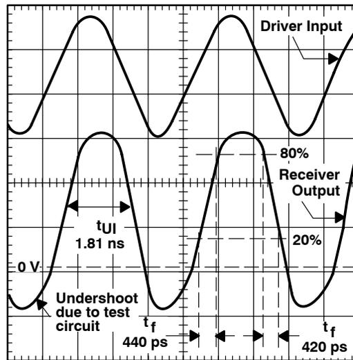
**Figure 3. Typical Signals at the Maximum Signaling Rate**
