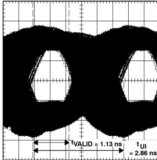
**Figure 4. Overlay of Four Receiver Outputs of a 16-Circuit Random Data Transfer**
