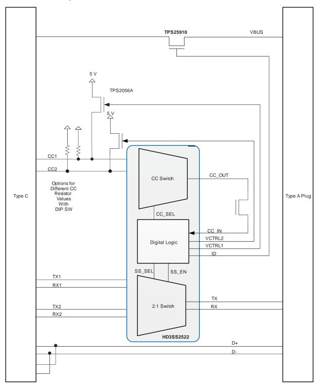
Figure 2. HD3SS2522 EVM Block Diagram
