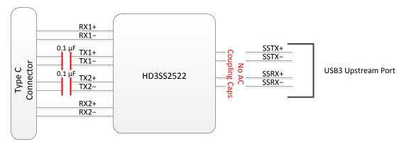
Figure 4. HD3SS2522 USB Upstream Implementation Example With 0 V < SSTX/RX Vcm < 2 V
