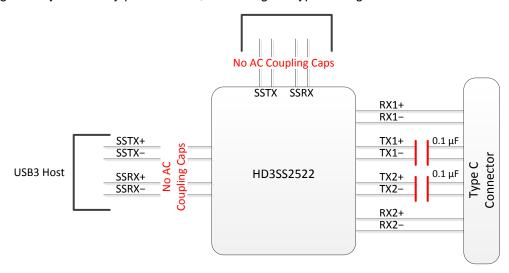
Figure 3. HD3SS2522 USB Host Implementation Example With 0 V < SSTX/RX Vcm < 2 V
