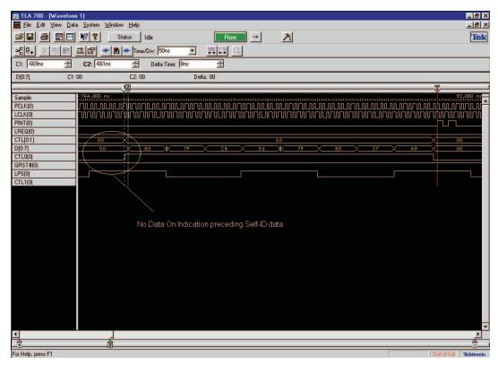
Figure 4. PHY/LINK Interface After Bus Reset With TSB41BA3DI / TSB41BA3D
