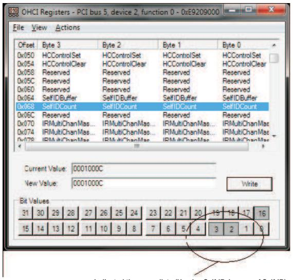
Indicated three quadlets (Header, Self-ID, Inverse of Self-ID) of Self-ID data present in host memory.
