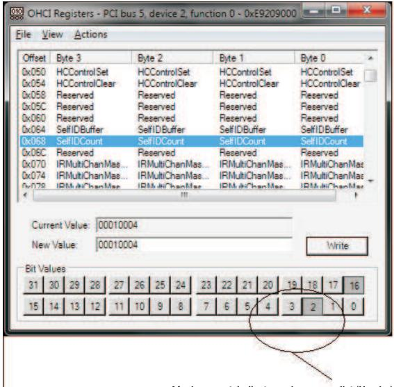
Afer bus reset, indicates only one quadlet (Header) of Self-ID information in host memory.
