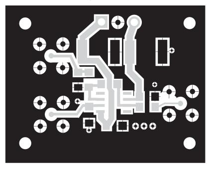
Figure 2-3. THS4051 EVM PC Board Layout - Back Side
