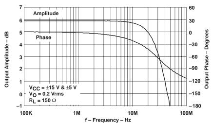
Figure 1–3. THS4051 EVM Frequency Response With Gain = +2
