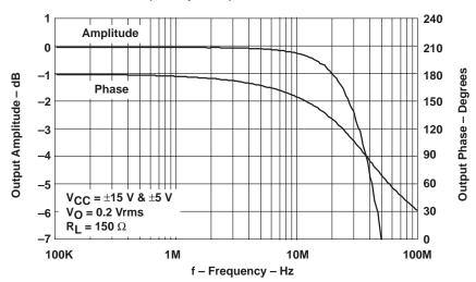
Figure 1-4. THS4051 EVM Frequency Response With Gain = -1
