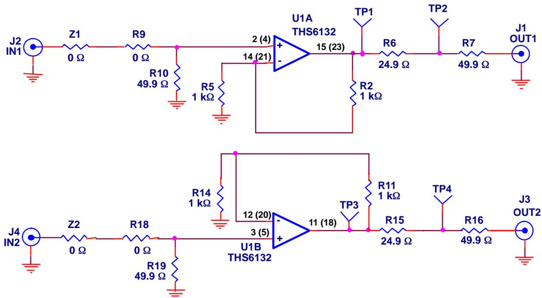
**Note:** Component pin numbers shown are for THS6132RGW while pin numbers in parentheses are for THS6132VFP.
