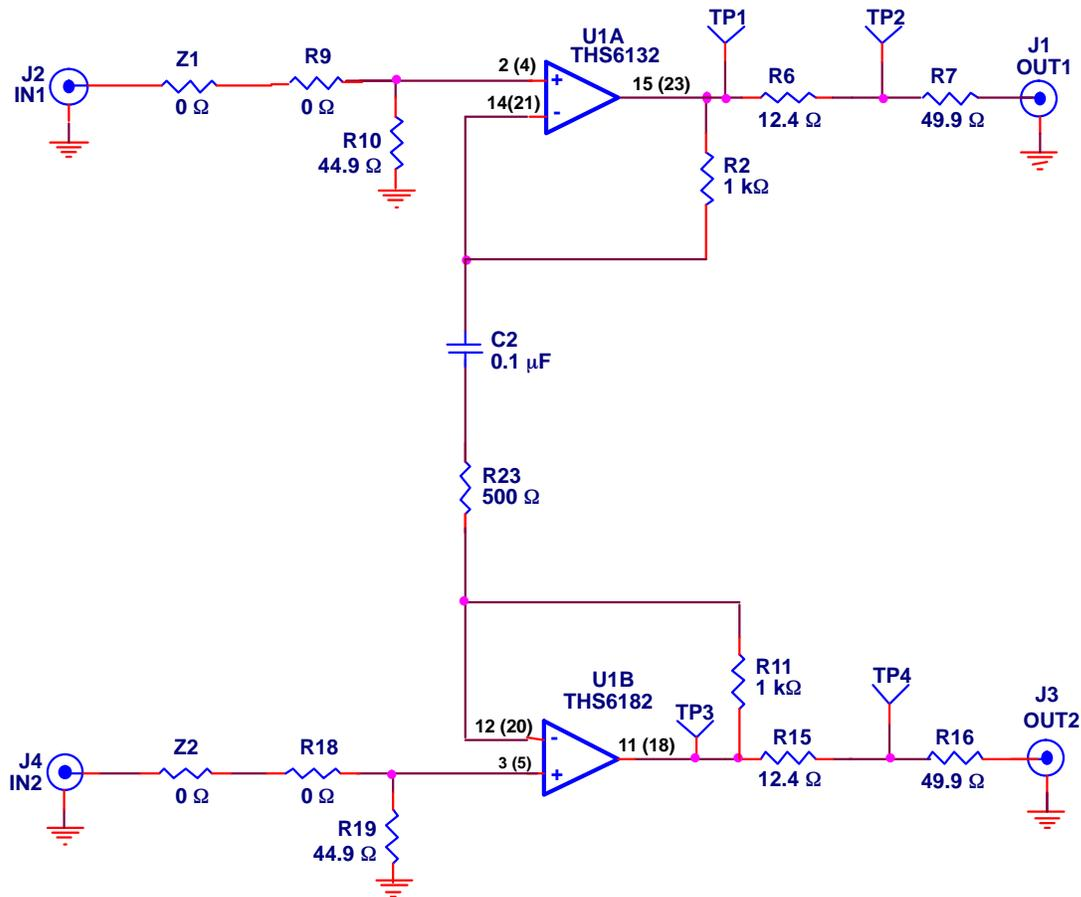
**Note:** Component pin numbers shown are for THS6132RGW while pin numbers in parentheses are for THS6132VFP.
