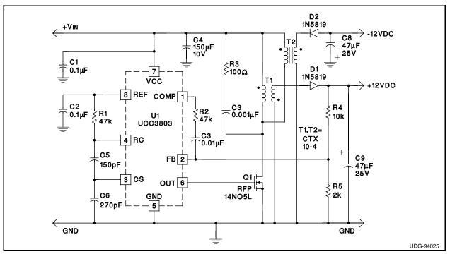
Figure 1. +5 to ±12V/80mA Converter
