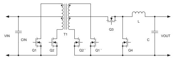
Figure 1. Push-Pull Converter Using Synchronous Rectification Followed by a Buck Regulator
