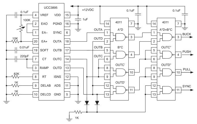
Figure 5. Circuit Implementation Using NAND Gates
