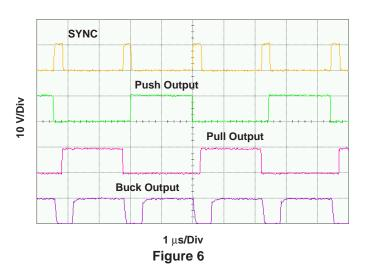
FUNDAMENTAL TIMING WAVEFORM
