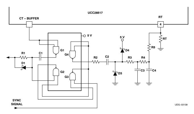
Figure 1. Synchronization Circuit for the UCC28517
