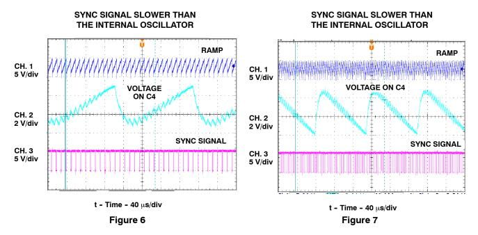
The filter consisting of R3–C3 was set with a 3 dB point at a factor of about 6 below the internal ramp frequency. In this case the ramp frequency was 100 kHz and the filter was set at about 25 kHz with a 6.1-k $\Omega$  resistor and a 1-nF capacitor. The second filter R5–C5 has to have a much higher impedance than the first to limit the influence on the first so a 25-k $\Omega$  resistor and 100-pF resistor with a filter 3 dB frequency of 60 kHz was used.
