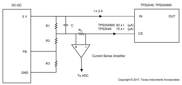
Figure 3. Current-Sensing Scheme With CS Pin
