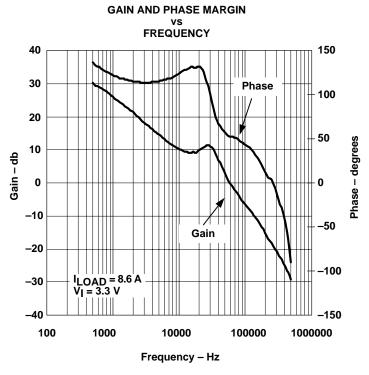
Figure 2. Gain and Phase Plot with 2.2-A Load
