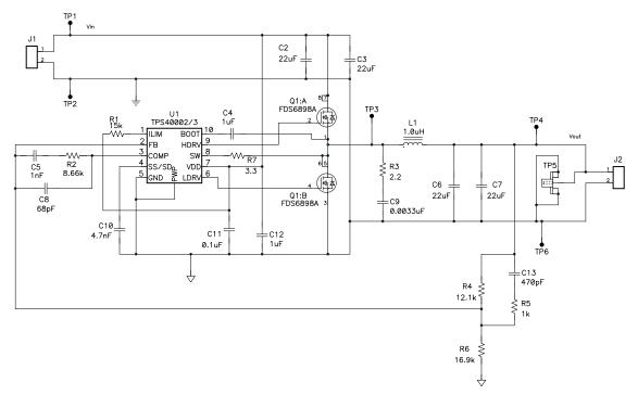
Figure 1. Application Diagram for the TPS40002/3
