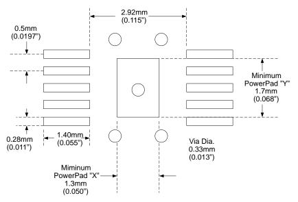
Figure 3. PowerPAD PCB Layout Guidelines
