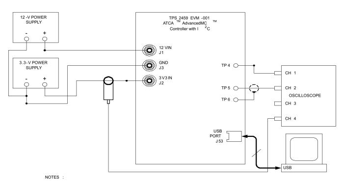
Run separate leads from the GND jacks back to a common return point made near the power supply output terminals
