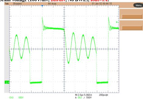
Ch3: Q1 Drain voltage (100V/div, 2us/div, No BWL), Iout=1A.
