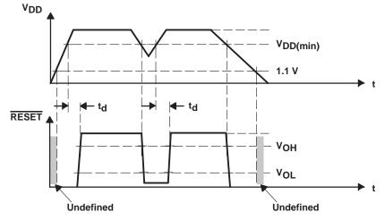
Figure 5. Timing Diagram of V<sub>DD</sub> and RESET Output
