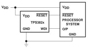
Figure 9. TPS382x System using WDI
