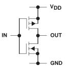
Figure 12. CMOS I/O Structure
