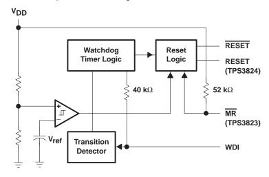
Figure 3. Simplified Block Diagram
