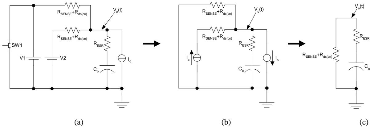
**Figure 3. OR-ing Circuit Electrical Model**
