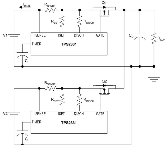
**Figure 2. An OR-ing Circuit for Two Power Supply Modules**
