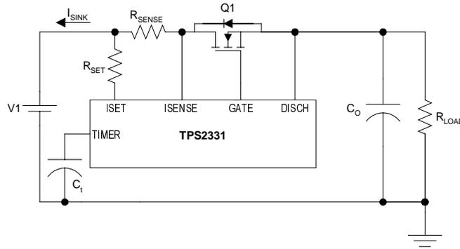
**Figure 1. Simplified Diagram of a Hot-Swap Circuit**
