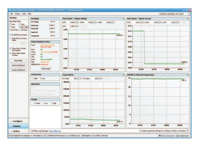
Figure 12. Rail #1 Voltage and Current Measurements
