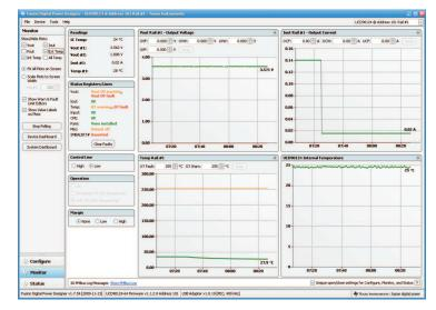
Figure 14. Rail #1 – Voltage, Current and Temperature Measurements
