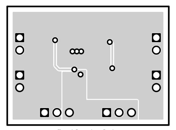
Figure 8. Bottom Layer Routing
