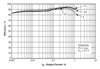
Figure 4. Efficiency Over Li-Ion Cell Range
