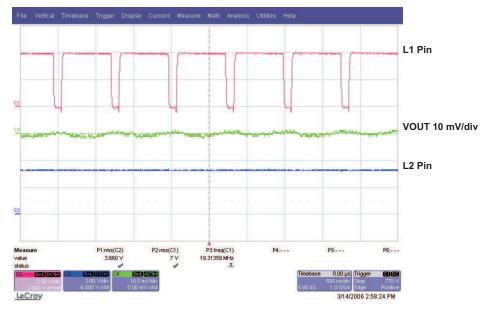
Figure 3. Output Ripple Vin 4.0 V
