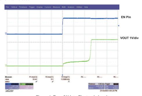
Figure 1. Turn ON into Electronic Load
