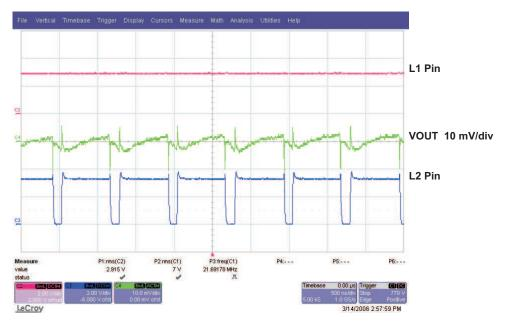
Figure 2. Output Ripple Vin 3.0 V
