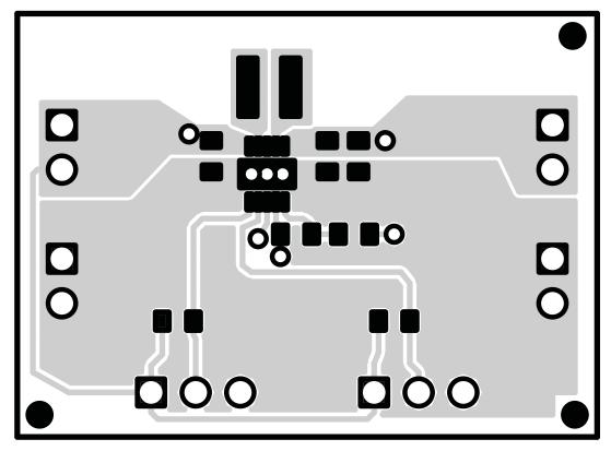
Figure 7. Top Layer Routing
