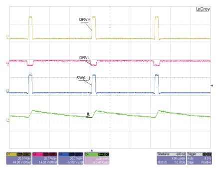
$V_{IN} = 20 \text{ V}, I_{OUT} = 4 \text{ A}, SW2 = 350 \text{ kHz}$
