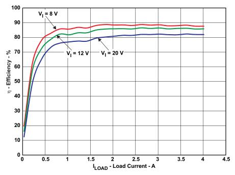
$V_{IN} = 8 \text{ V} - 20 \text{ V}, V_{OUT} = 1.20 \text{ V}, I_{OUT} = 4 \text{ A}, SW2 = 350 \text{ kHz}$
