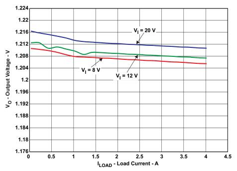
$V_{\text{IN}}$  = 8 V - 20 V,  $V_{\text{OUT}}$  = 1.20 V,  $I_{\text{OUT}}$  = 4 A
