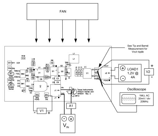
Figure 2. TPS53114EVM-541 Recommended Test Setup
