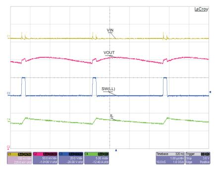
$V_{IN} = 20 \text{ V}, \ V_{OUT} = 1.20 \text{ V}, \ I_{OUT} = 2 \text{ A}, \ SW2 = 350 \text{ kHz}$
