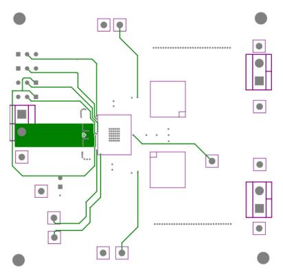
Figure 5. Board Layout (Third Layer)
