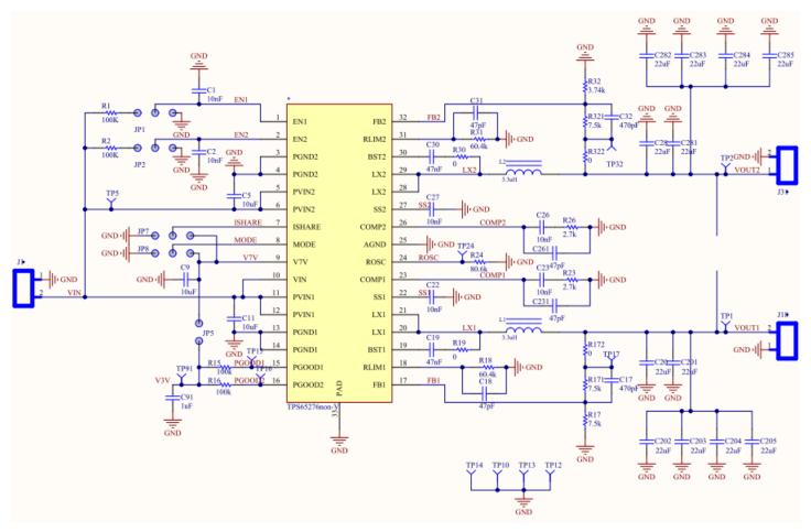
Figure 1. TPS65279 Schematic
