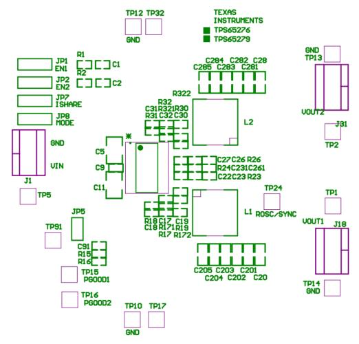
Figure 2. Component Placement (Top Layer)
