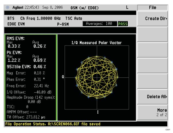
Figure 3. GSM EDGE EVM at 1800 MHz
