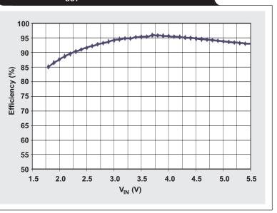
buck and boost functions into a single  $3 \times 3$ -mm QFN package, including switching FETs, compensation, and protection features. Only three external parts are required for operation: input and output capacitors and an inductor. The converter operates with a peak efficiency of 96% (see Figure 1). With a peak output current of 800 mA, it delivers
