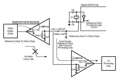
Figure 5. Implementing the LMV112 to Reduce Clock Circuit Interaction
