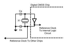
Figure 3. Reference Clock Circuit Inside a Digital CMOS Chip
