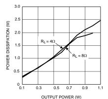
Figure 10. Power Dissipation vs Output Power  $V_{cc} = 3.3V$
