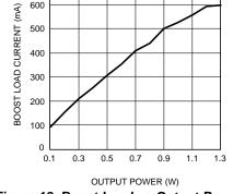
Figure 18. Boost Load vs Output Power  $V_{\text{DD}}$  = 4.2V,  $R_{\text{L}}$  = 8 $\Omega$
