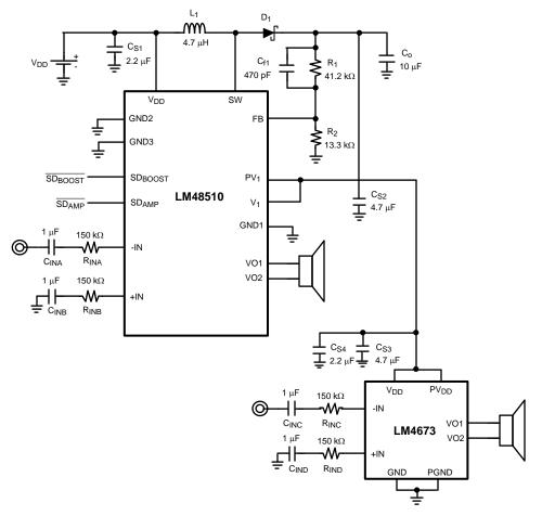
Figure 1. LM48510 Stereo Typical Application
