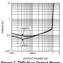
Figure 7. THD+N vs Output Power  $V_{cc} = 3.3V$ ,  $V_1 = 5.0V$ ,  $R_L = 15\mu$ H+8 $\Omega$ +15 $\mu$ H 22kHz BW
