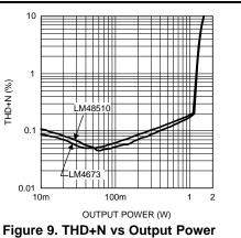
Figure 9. THD+N VS Output Power  $V_{cc} = 4.2V, V_1 = 5.0V, R_L = 15\mu H+8\Omega+15\mu H$ 22kHz BW
