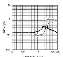
$\label{eq:FREQUENCY (Hz)} \begin{array}{l} \mbox{Frequency (Hz)} \\ \mbox{Figure 3. THD+N vs Frequency} \\ \mbox{V}_{cc} = 3.3V, \mbox{V}_1 = 5.0V, \mbox{R}_L = 15\mu H{+}8\Omega{+}15\mu H \\ \mbox{P}_o = 500mW, \mbox{22kHz BW} \end{array}$
