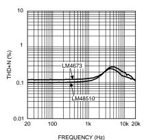
Figure 5. THD+N vs Frequency  $V_{cc} = 4.2V, V_1 = 5.0V, R_L = 15\mu H+8\Omega+15\mu H$  $P_o = 500 mW, 22 kHz BW$
