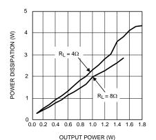
Figure 11. Power Dissipation vs Output Power  $V_{cc}$  = 4.2V
