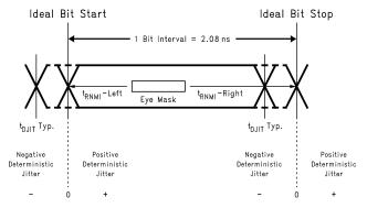
Figure 3. Parameter Relationships to Generate the Eye Mask
