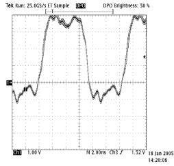
With 24 mA of drive programmed into the FPGA outputs, large excursions outside the supply rails are clearly visible.
