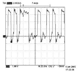
Figure 7. 24 mA FPGA Output +4" Trace with PRBS Data
