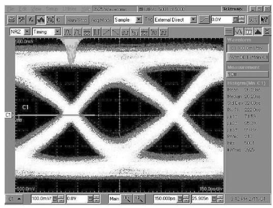
Measured after 15m of Infiniband Cable at the Input of the DS92LV18 Receiver; f<sub>TCLK</sub> = 66 MHz (1.32 Gbps); Max Pre-emphasis
