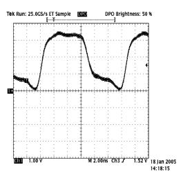
Reducing the FPGA programmed drive to 2 mA results in a tightly controlled clock waveform.
