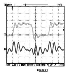
Figure 4. Active Output Transitions and "Quiet Output" (bottom), SS Data, 24 mA
