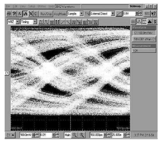
Measured after 15m of Infiniband Cable at the Input of the DS92LV18 Receiver;  $f_{TCLK}$  = 66 MHz (1.32 Gbps); No Preemphasis
