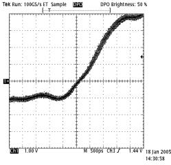
Rising Edge Magnification: This view shows greater than 200 ps of clock jitter in the FPGA output that is a result of the increased drive current.
