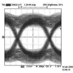
Figure 9. Eye Diagram after 1m of CAT5 Cable
