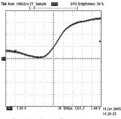
Rising Edge Magnification: This view shows how a reduced 2 mA drive current maintains good signal integrity and exceptionally low (~50 ps) jitter.
