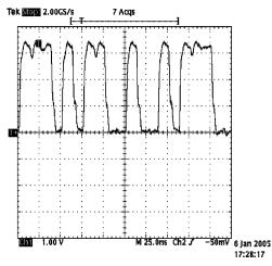
Figure 8. 2 mA FPGA Output +4" Trace with PRBS Data
