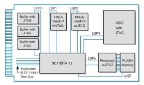
Figure 1: Typical Use of SCANSTA112 for Board Level Management of Multiple JTAG Chains
